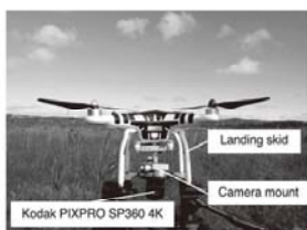
Fig. 2. UAV system equipped with omnidirectional movie camera.
